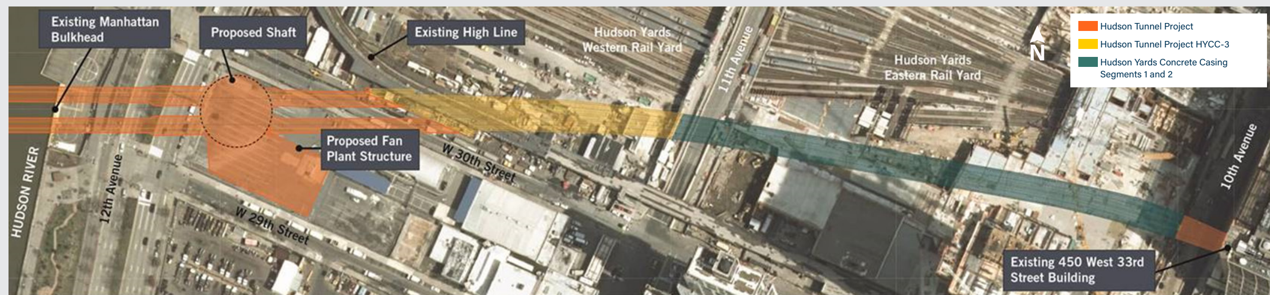
Figure 1-7 Hudson Tunnel Project – Manhattan Tunnels
