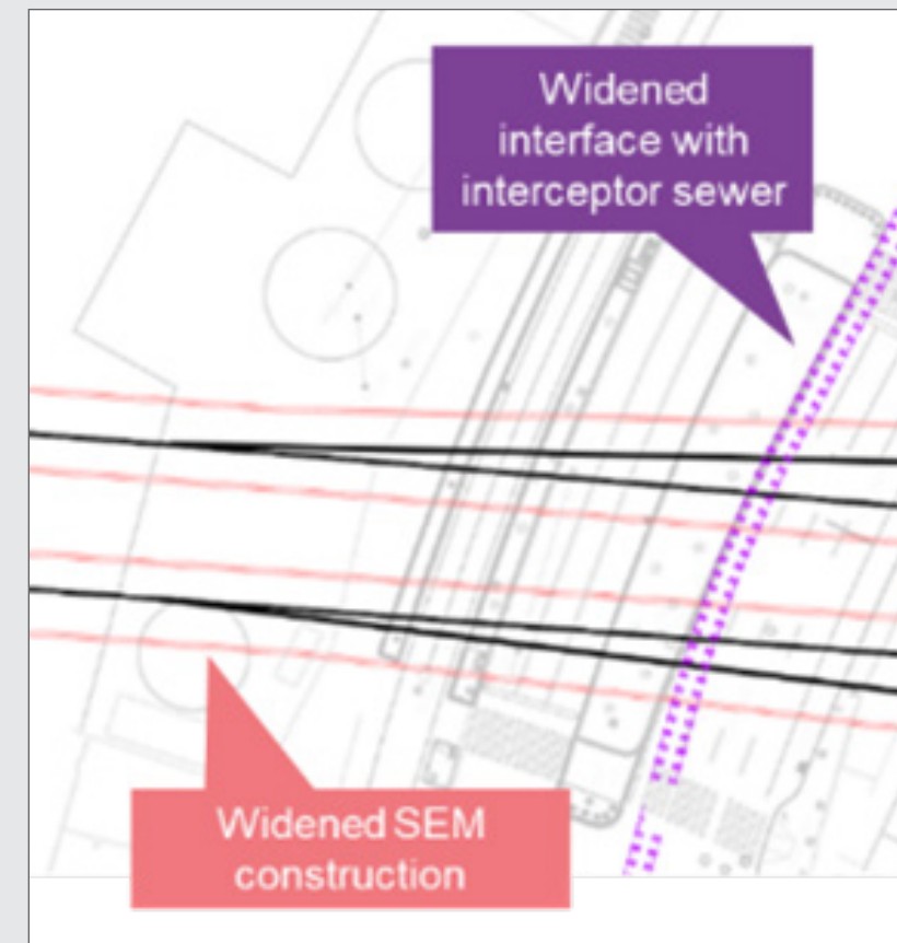
Figure 5-5 Interface with Twelfth Avenue Interceptor Sewer
