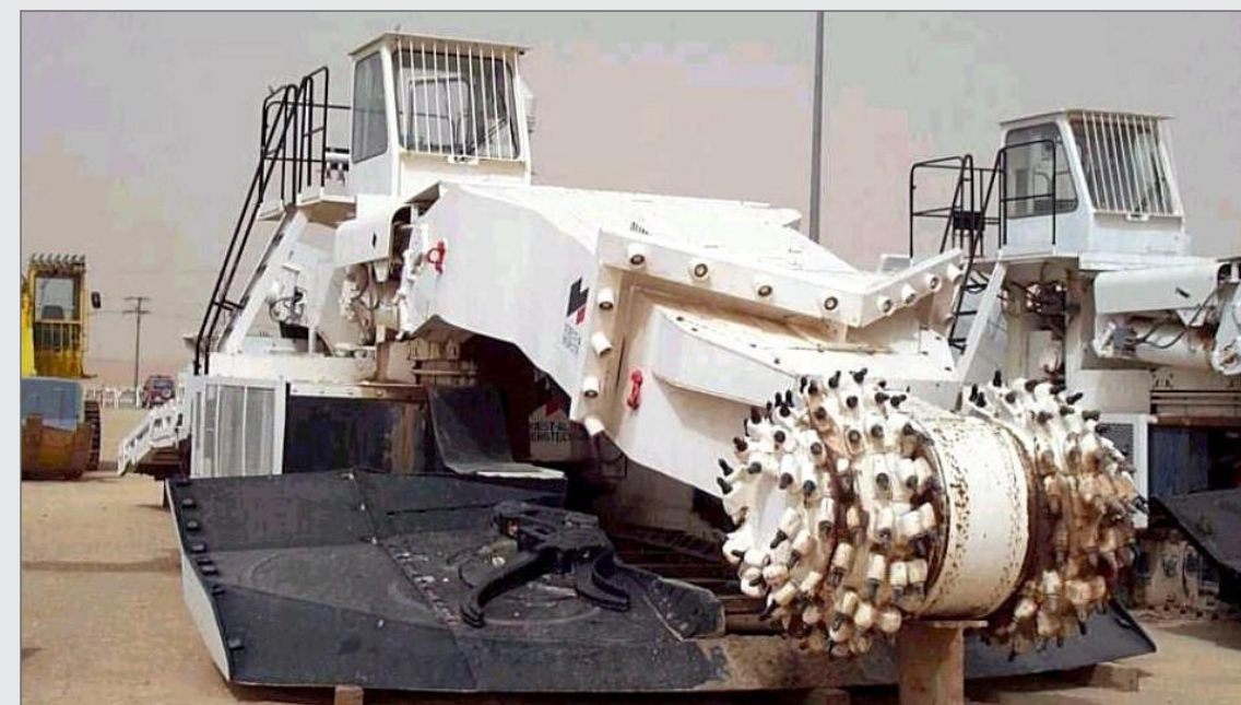
Figure 4-24 Roadheader Excavation Machine
